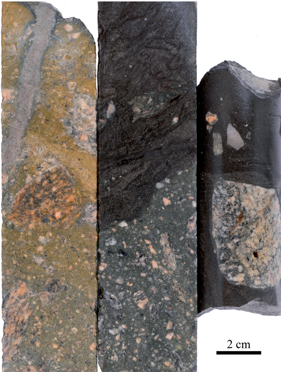
Figure 10. Three core samples of the Mesozoic Bjarøy Formation. Left: Breccia, interpreted as sedimentary, with sand vein (top). Middle: transition from grit to quartz-rich sandstone with a few small coal fragments. Right: sandstone with gneiss fragments. These and other samples from the Bjarøy tunnel in West Norway are part of the Natural History Collections at Bergen Museum, University of Bergen.
